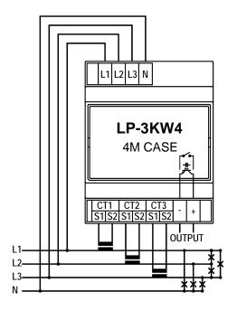
Output open collector opto coupler or relay
