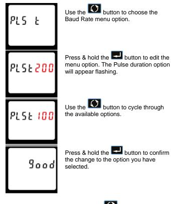
To exit the set-up menu, press & hold O until the measurement screen is restored.
