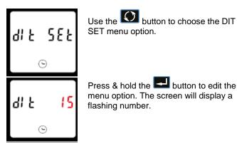
Use the button to cycle through the available options. <u> ፈነ ኑ</u> Θ Press & hold the 🛃 button to confirm the change to the option you have 9000 selected.
