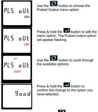
To exit the set-up menu, press & hold the measurement screen is restored.
