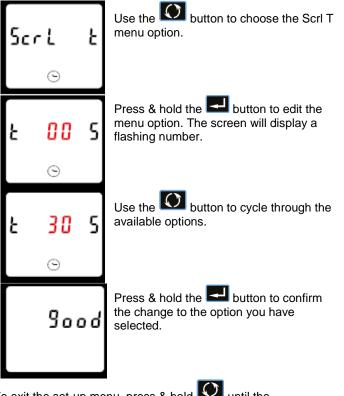
To exit the set-up menu, press & hold 🚺 until the measurement screen is restored.
