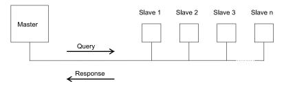
In the MODBUS™ Protocol the master can address individual slaves, or, using a special "Broadcast" address, can initiate a broadcast message to all slaves. The DRS-100-1P digital MID Energy Meter does not support the broadcast address.
