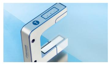
With a fork width of only 30 mm and 60 mm respectively and a depth of 33 mm and 73 mm respectively, it has a very compact design. Its working range of 12 mm and 40 mm respectively and its high accuracy of 0.1 mm permit a wide variety of applications.
