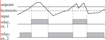
Example 1, undervoltage monitoring pin 6-7 not connected
