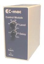
C-mac<sup>®</sup> monitoring relay, type RM34, is used for temperature metering in conjunction with Pt100 temperature sensors according to DIN 43760. A 3-wire metering principle is used, which means that the module compensates for the external cable resistance. The cable monitoring circuit also ensures that the relay will release in case of short-circuit or cable breakage.
