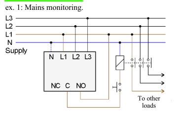
When the monitoring relay is connected as shown on the drawing above, the mains supply must be correct, before the load can be activated. This is particularly important if the load is sensitive to under- or over-voltage, and to ensure correct rotation direction of motors. This monitoring principle is recommended, when you want a general monitoring of the mains supply to several loads at the same time.
