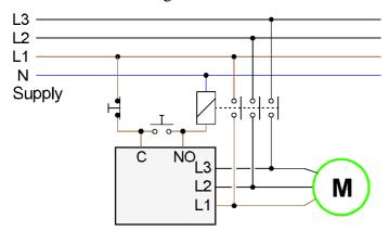
If instead you want to monitor the supply voltage for a single load, you can connect the monitoring relay after the contactor, in this way the contactor itself is also monitored. This principle is recommended if f.inst. you want a quick reaction in case of a phase failure to a motor. In the example above, the relay output is connected in parallel with the start contact, thereby it latches the contactor, if the supply is OK and in case of an error, the contactor is released.
