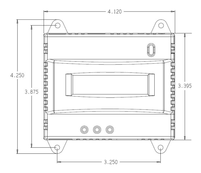
The AcuLink 710 has 4 mounting holes for use with a #6 screw. The drawing above shows the relative position of the mounting holes.
