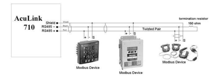
**Step 4** - Power-up and diagnostics: A power supply is not provided with the AcuLink 710, therefore it is up to the installer to provide the required 24VDC. After power is applied, the green "Alive" light in the upper right of the AcuLink 710 should come on and the LCD display will display a series of diagnostic screens ending with the following message on the LCD display (this boot sequence may require up to 20 seconds to complete):
