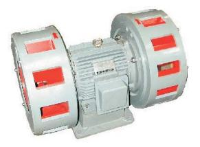
The Carrel & Carrel double ended 3-phase siren is designed to give effective warning over wide areas. The unit has the typical air raid siren sound, the low frequency giving excellent sound coverage. The siren is designed for roof, pole, tower or plinth mounting. Its construction ensures long life. The siren is powered by a 4kW 3-phase motor and is continuously rated.
