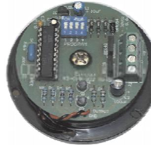
The EWS 6 is a digitally based electronic sounder housed in a self contained horn speaker and has 16 separate tones selected on a 4 way DIP switch on the internal pc board.
