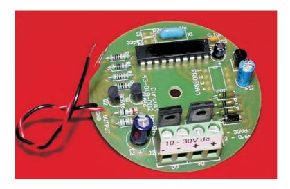
The Carrel-Electrade EWSF-PCB driver board can be easily installed into most standard fire alarm horns giving a true AS2220 evacuation tone.
