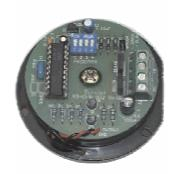
The EWS 6 is a digitally based electronic sounder housed in a self contained horn speaker and has 16 separate tones selected on a 4 way DIP switch on the internal pc board.
