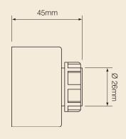
A compact sounder, purpose designed to fit through the fascias of control panels or equipment housings. The single nut fixing ensures simple installation and maximum audibility, while the high IP rating allows installation in most process and industrial environments.
